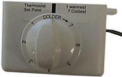
The OFF position is reached by turning hard counterclockwise past the click. The reference point is shown with an indicator sticker beside the knob.
