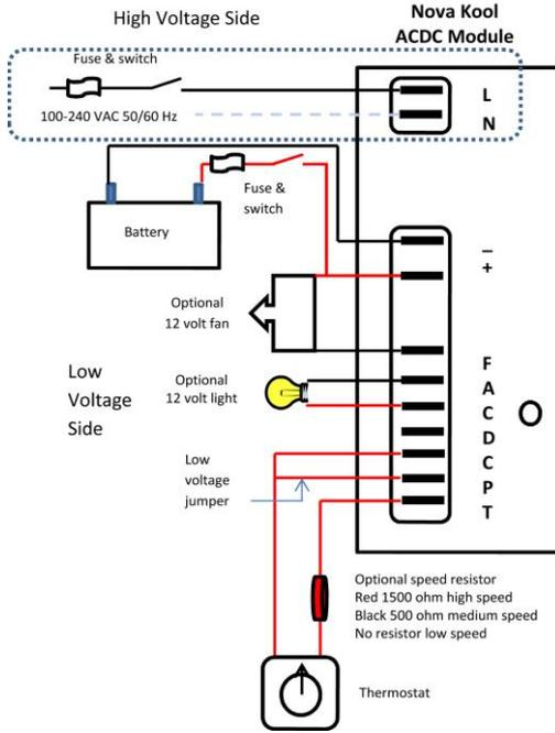
After Serial number 256409 the thermostat wire has an additional green or red wire which is used to control cut out voltage. If it is placed on P the cut out voltage is 9.4 vdc if it is simply left off of terminal P the cut our voltage is 10.6 vdc.
